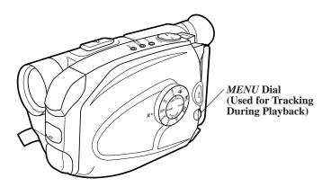
During playback, streaks may appear in the playback picture. Press the *MENU* dial in to activate manual tracking. Rotate it up or down to move the streaks up or down and out of the picture.
